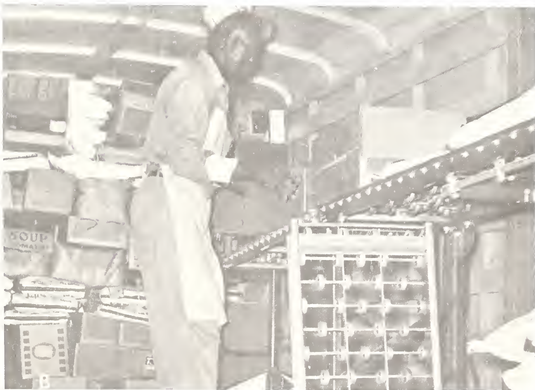
FIGURE 6.—Conveyor systems in use in wholesale grocery operations for A, receiving and B, truck loading.
