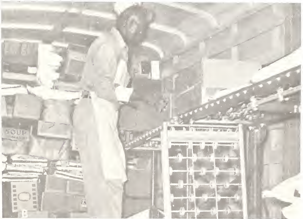
FIGURE 6.—Conveyor systems in use in wholesale grocery operations for A , receiving and B , truck loading. BN-3131, BN-3142
