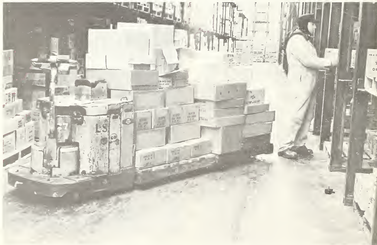
FIGURE 3.—A pallet jack that handles two pallets, used to select frozen food orders.
