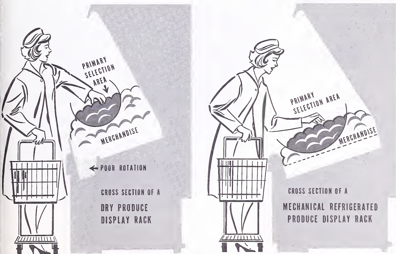
Figure 8.--Cross section drawing of typical produce display counter bases showing the area of primary selection available to the customer.
