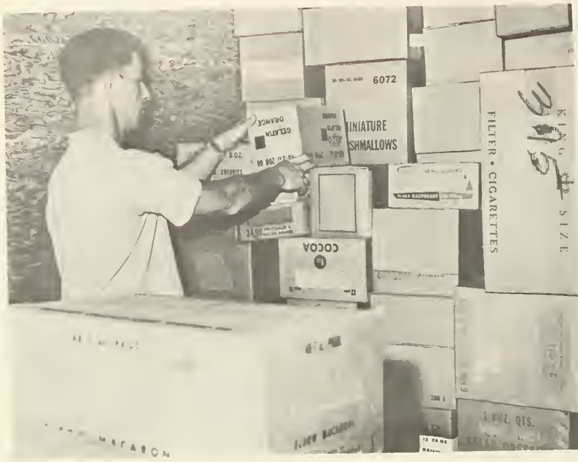
Figure 5.--Handstacking cases assembled without pallets. Cases are handstacked from the selector truck, which is pushed into the trailer.
