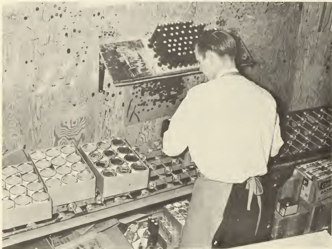
Figure 15.--Price-marking in the grocery storeroom, using the half case method. This work surface is at a convenient height and the stamps readily accessible. When stamps are not in use, the inclined shelf is raised to a horizontal position to insure even distribution of ink in the stamp-set base.
