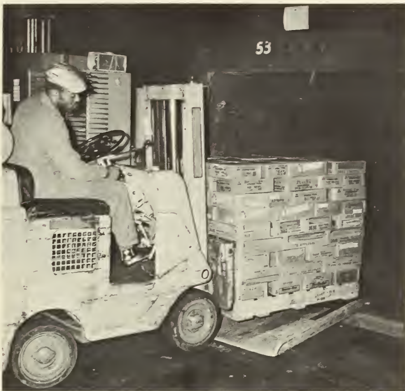
Figure 4.--Using a low-mast forklift truck to load palletized orders into a trailer. The trailer floor must be strong enough to support the weight of the loaded forklift truck.
