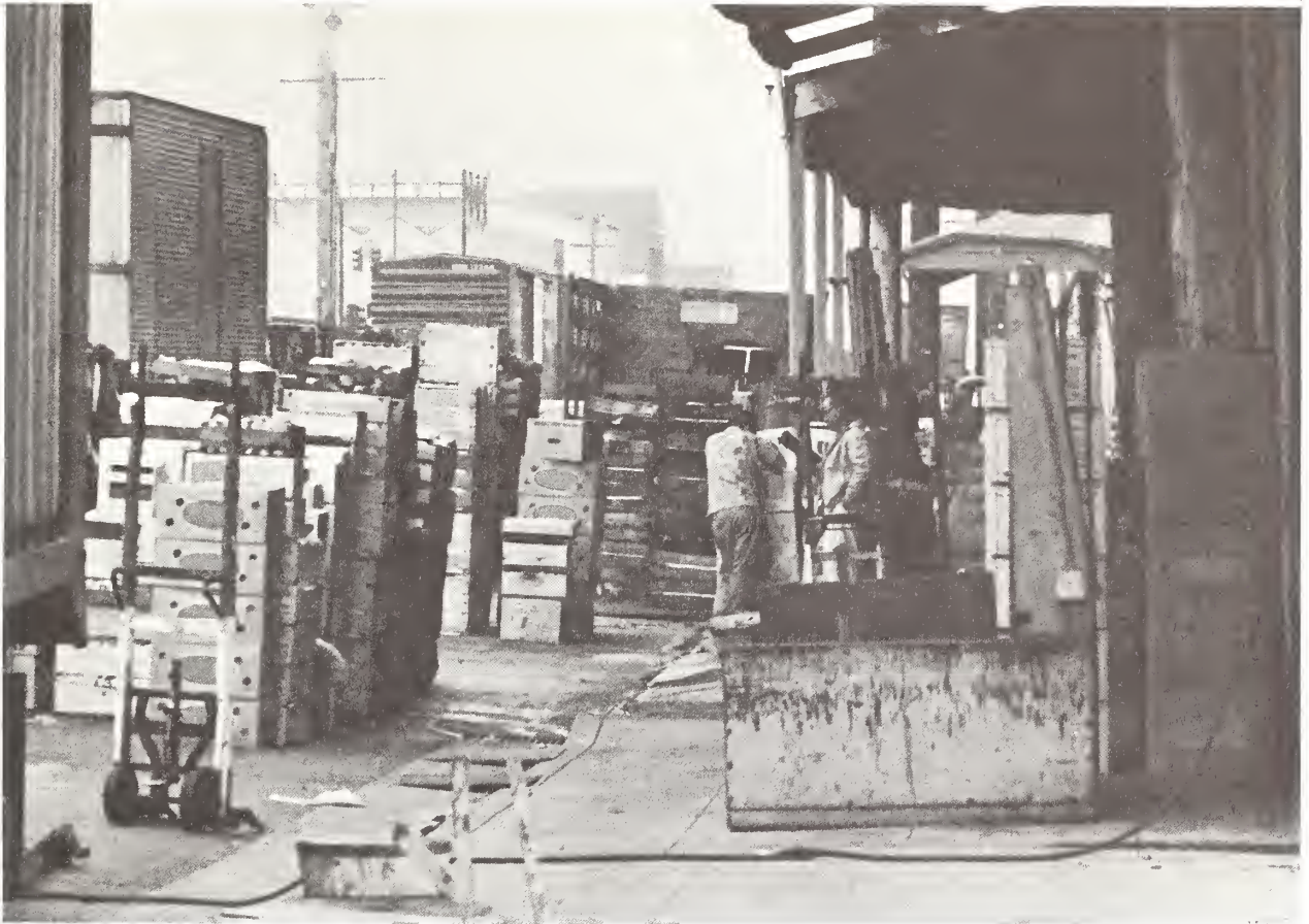
FIGURE 6.—Lack of platform space in most food related facilities forces loading and unloading directly in the street, causing confusion and additional handling.
