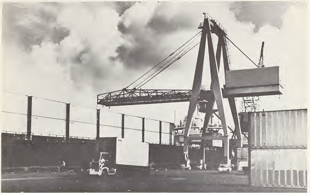
FIGURE 2.--Diamond Head Terminal: Containers being unloaded by large gantry cranes at pier 2.
