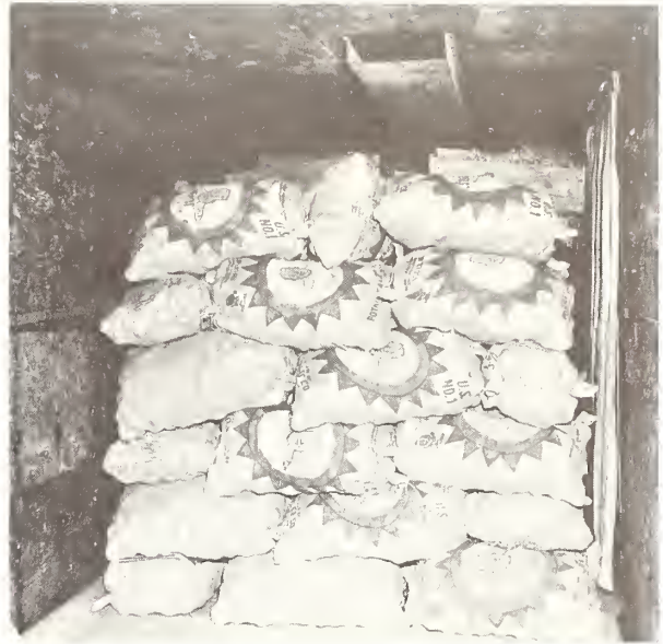
Figure 3.--Solid-load pattern with wool spoce, for bagged potatoes in semitrailers. Note outlet, at ceiling level, for air delivery from blower-fan.
