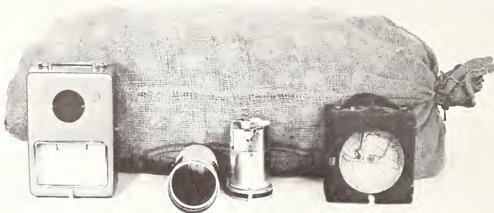
Figure 1.--Instruments for recording temperature data: 1, 10-hour recording thermometer for floor-level air temperature; 2, 30-day recording thermometer for inside-bag potato temperature; 3, 7-day recording thermometer for outside air transit temperature.
