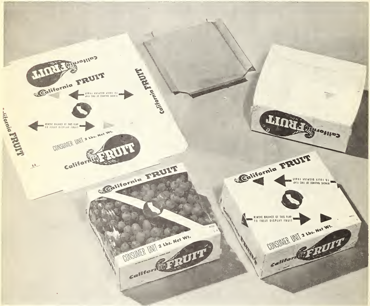
Figure 1.--This is the window carton with recessed bottom. The flat (upper left) is folded to form body of carton (upper right). After filling, the bottom (upper middle) is stapled in. The film window is covered with protective paperboard (lower right) which is removed when the carton is put on display (lower left).
