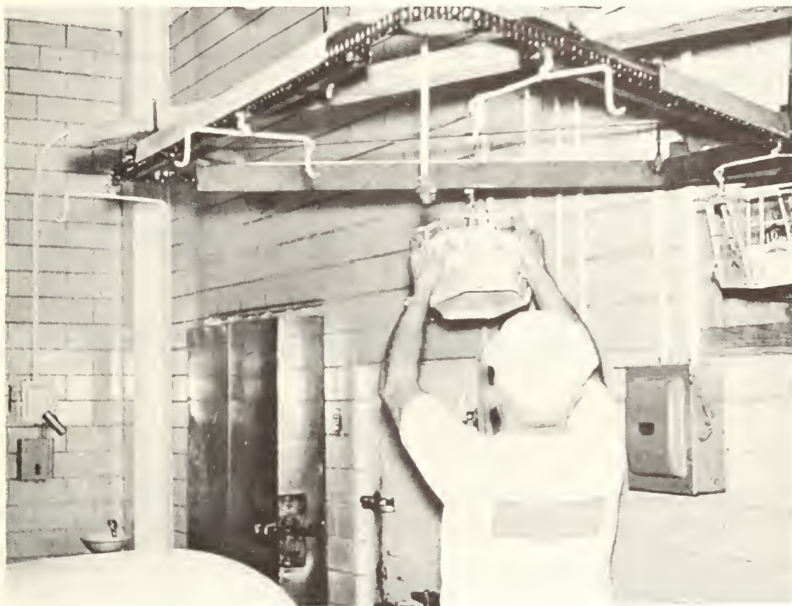
Figure 5.--The operator of filling machine hitches full case of tetra containers to ingenious overhead conveyor which will carry them to refrigerator.
