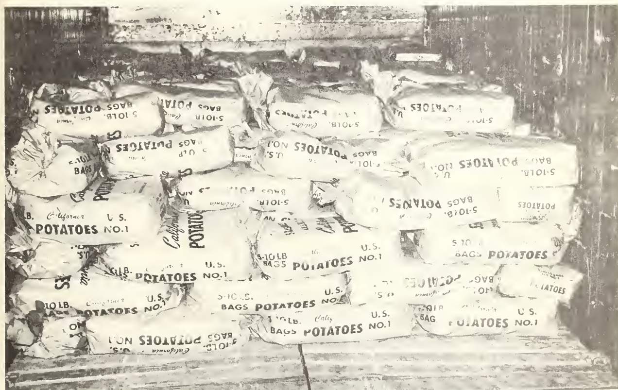
Figure 5.--Cross section view of railway car loaded with paper master containers; each container holding five 10-pound polyethylene bags.
