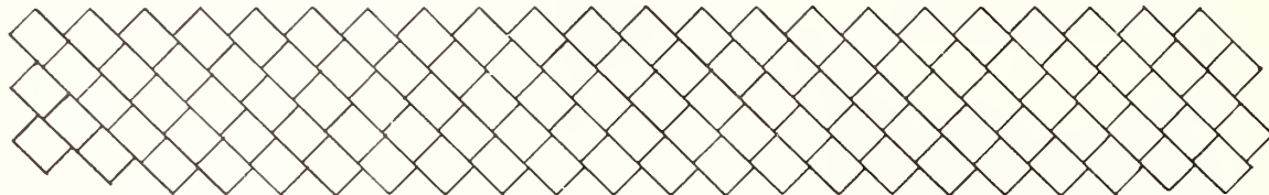
45° ANGLE STORAGE-44 FACINGS-110 PALLETS ON FLOOR
