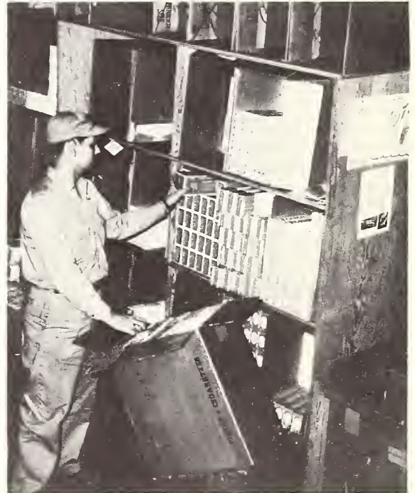
Figure 32.--An improved method of cigarette assembly with use of a rack and stool.
