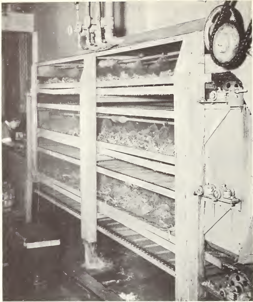
Figure 8.--Spinach passing through three layers of a spray washer in a final effort to remove all sand and grit.
