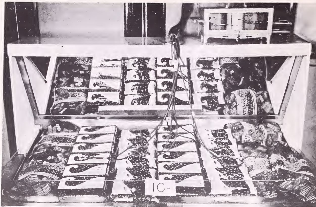
Figure 4. --Package arrangements and locations of the dummy blocks in the iced display case. The overhead cable connected thermocouples in packages to the electronic temperature recorder. All methods of display were similarly arranged. The hygrothermograph above the case recorded display room temperatures and relative humidities.
