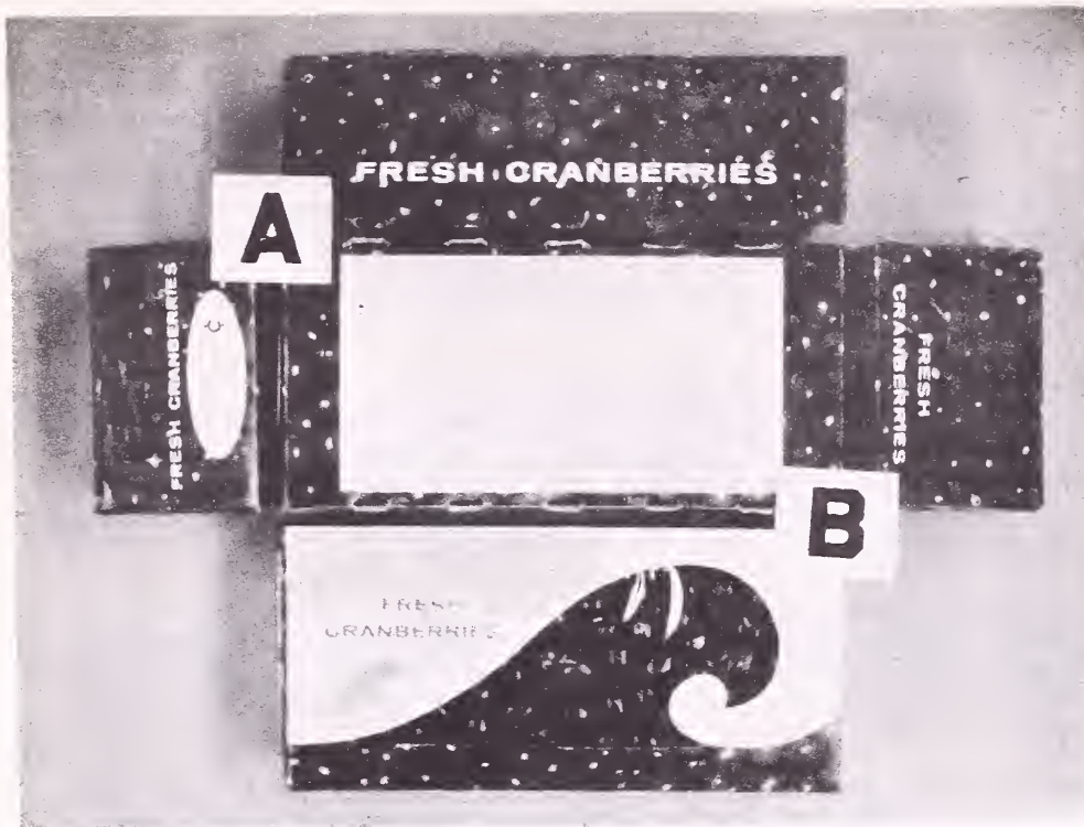
Figure 2.--Type of commercial box used in all experiments. Ten vents are located near points A and B on the longer bottom edges of the box.
