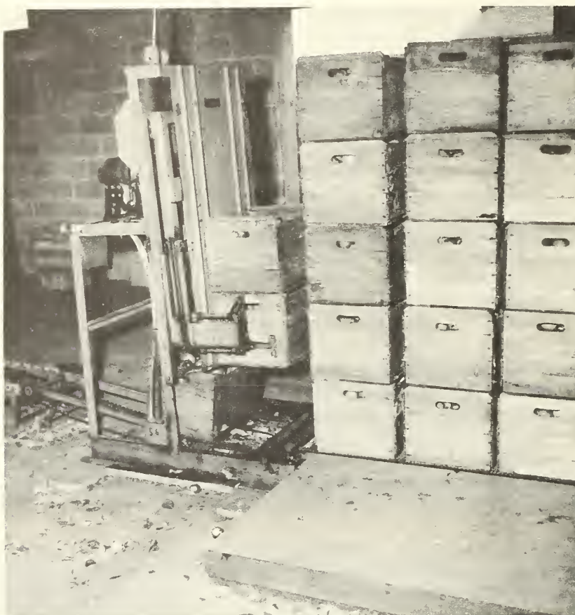
Figure 1.--Automatic de-stacker sometimes used in conjunction with the drum type, automatic dumpers.
