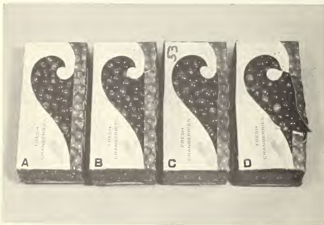
Figure 2. Different amounts of water damage that may occur to packages within 72 hours on various ice covers. Grades are identified as follows: (A) good = undamaged; (B) fair = slight damage, but salable; (C) poor = damaged, but salable at a discount; (D) very poor = damaged, completely water-soaked and unsalable without repackaging.
