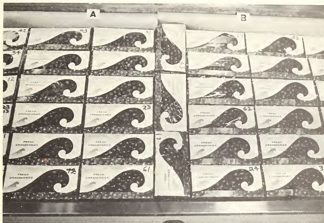
Figure 3. Polyethylene and kraft paper ice covers under test. The packages on the left, marked A, were on ice covered by a 2-mil sheet of polyethylene. The packages on the right, marked B, were on ice covered by heavy kraft paper. All B packages at the end of the test showed water marks and discoloration, while the A packages showed little or no damage.
