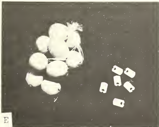
Figure 30.--Some methods of closing polyethylene bags: (a) Pressure-sensitive tape; (b) jaw-type hand stapler; (c) wire-enclosed paper tape; (d) metal clip; (e) plastic tag; and (f) saddle price tag and conventional stapler.
