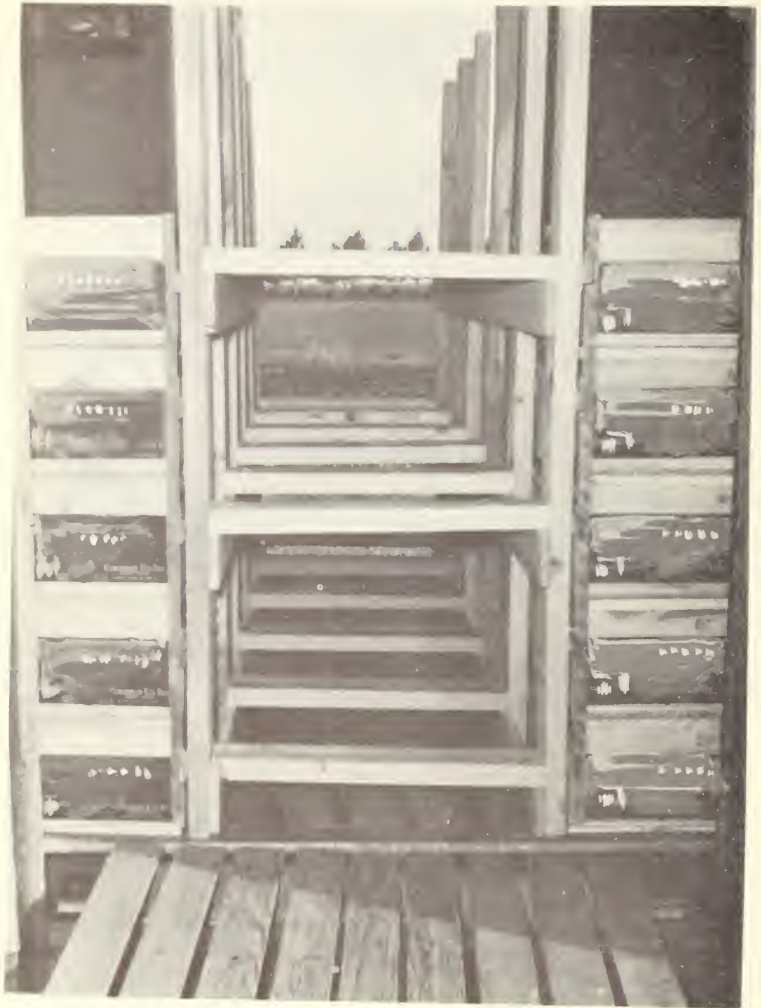
Figure 8.--Doorway view of a refrigerator carload of California tomatoes in 30-pound wooden lugs, showing center gate in place.
