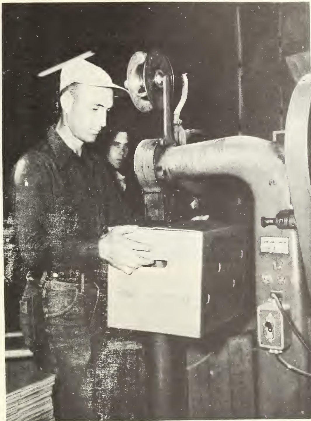
Figure 12.--Stitching flaps of one section of 50-pound full-depth telescope, dual-purpose fiberboard box.
