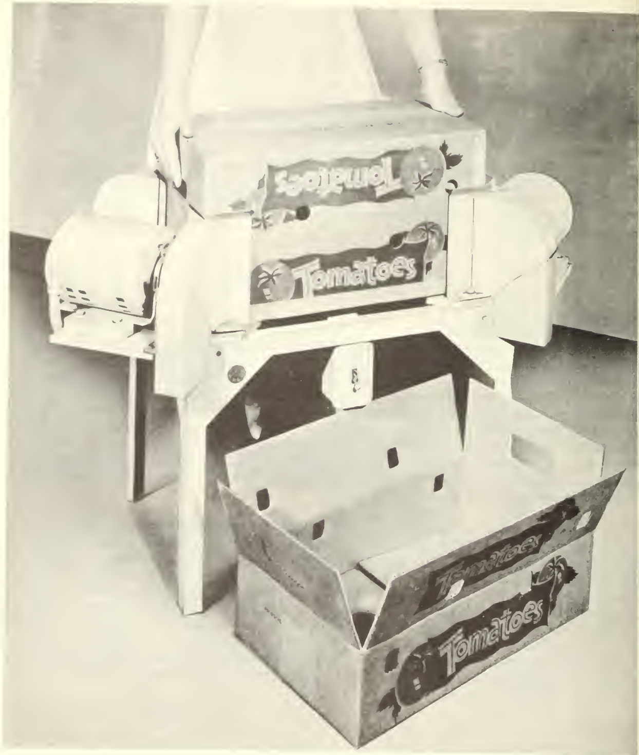
Figure 17.--One section of a 50-pound full-telescope, dual-purpose fiberboard shipping container being converted to a 20-tube master container.
