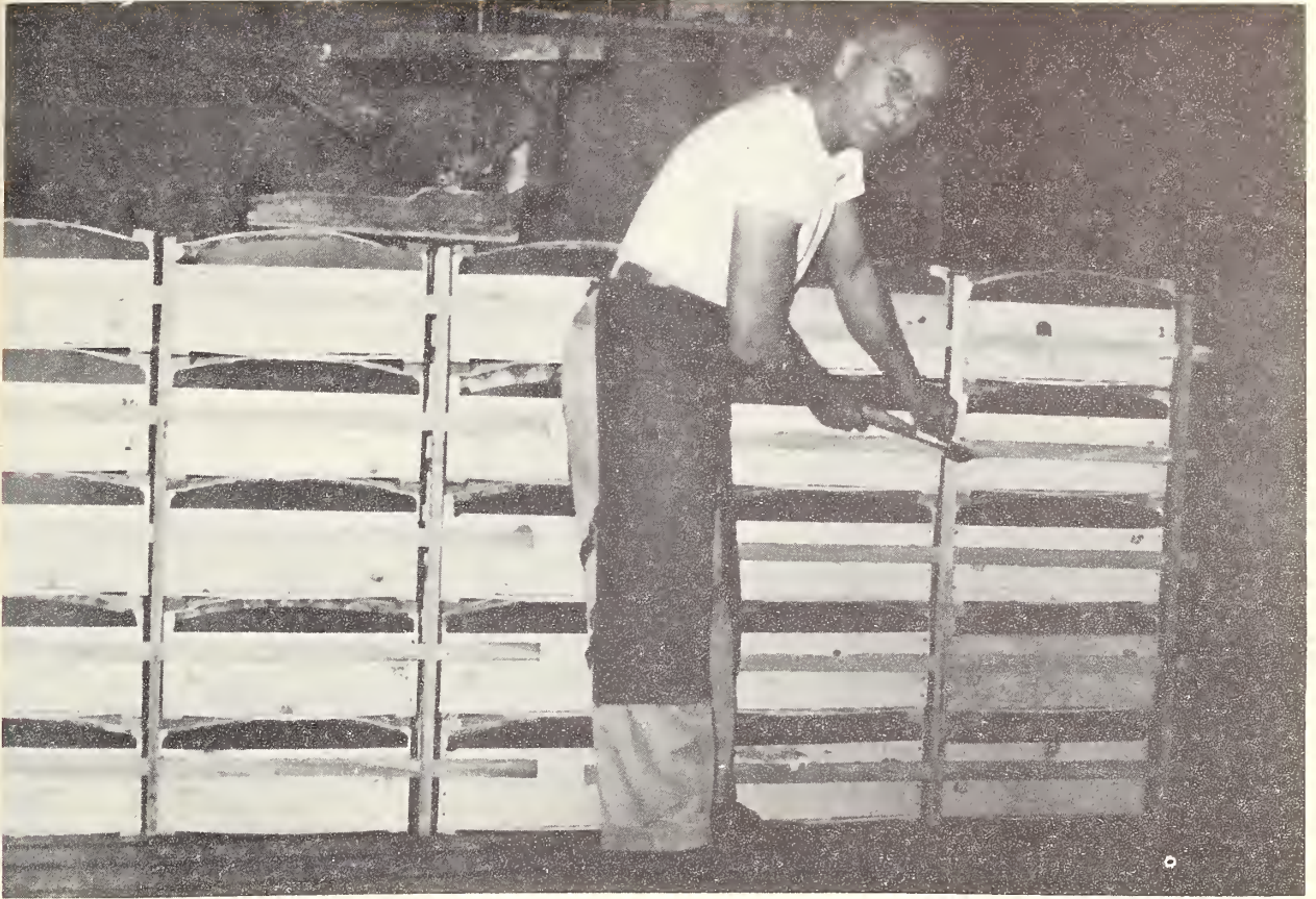
Figure 9.--Cross-section of a crosswise-on-bottoms load of 30-pound wooden lugs of California tomatoes, showing gate frames to hold lugs in row alignment being installed at the shipping point.
