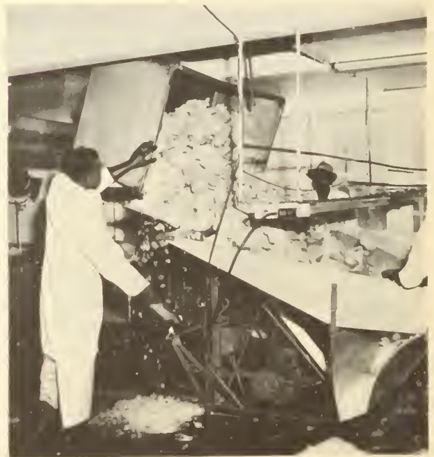
Figure 28. Tank tipper dumping tank of poultry onto improved packing table.
