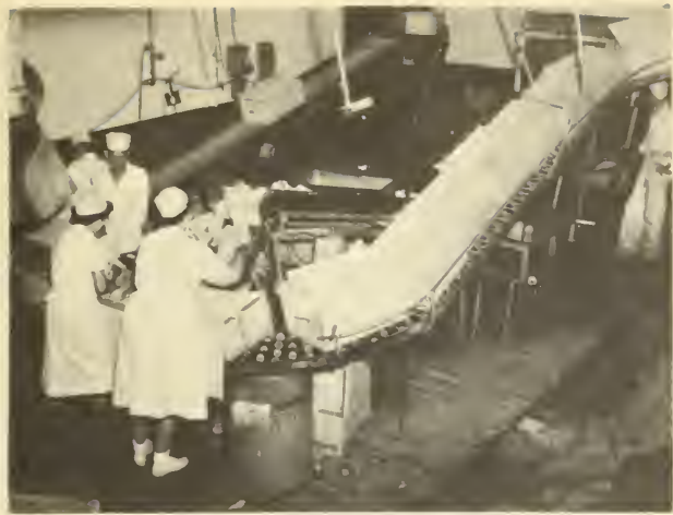
Figure 9. Transporting boxes to packing station by gravity chute.
