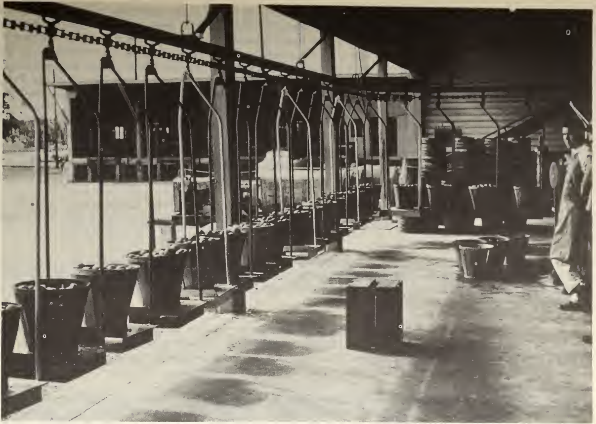
Figure 6. --Endless belt, cradle arrangement at Biglerville, Pa., for unloading hampers of tomatoes to be processed. Each cradle is painted 1 of 4 primary colors, in sequence, to facilitate efficient unloading of 4 vehicles at 1 time. A different color was assigned each vehicle and hampers of tomatoes were unloaded only on cradles of the same color.
