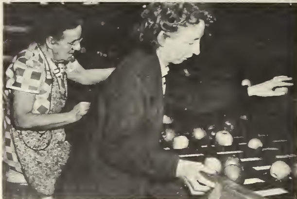
FIGURE 7.—Slightly higher speed of translation caused sorters to face toward the flow of the oncoming fruit.
