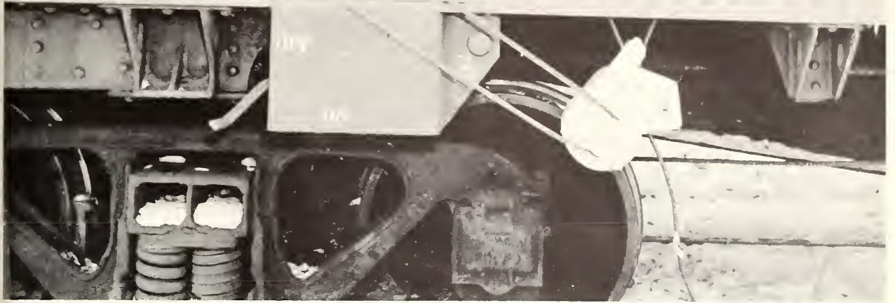
Figure 2.--Method of mounting electric motor to operate car fans while fans are standing on track.
