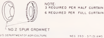
Figure 22.--Part No. 8 (grommet) used in making a curtain for use in a 30" x 64" door opening.
