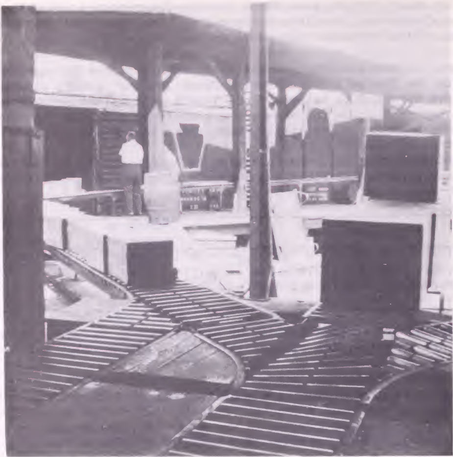
Figure 4.--A roller conveyor system used for receiving merchandise from rail cars and motor-trucks. Switches are used to direct merchandise to the proper floor level.
