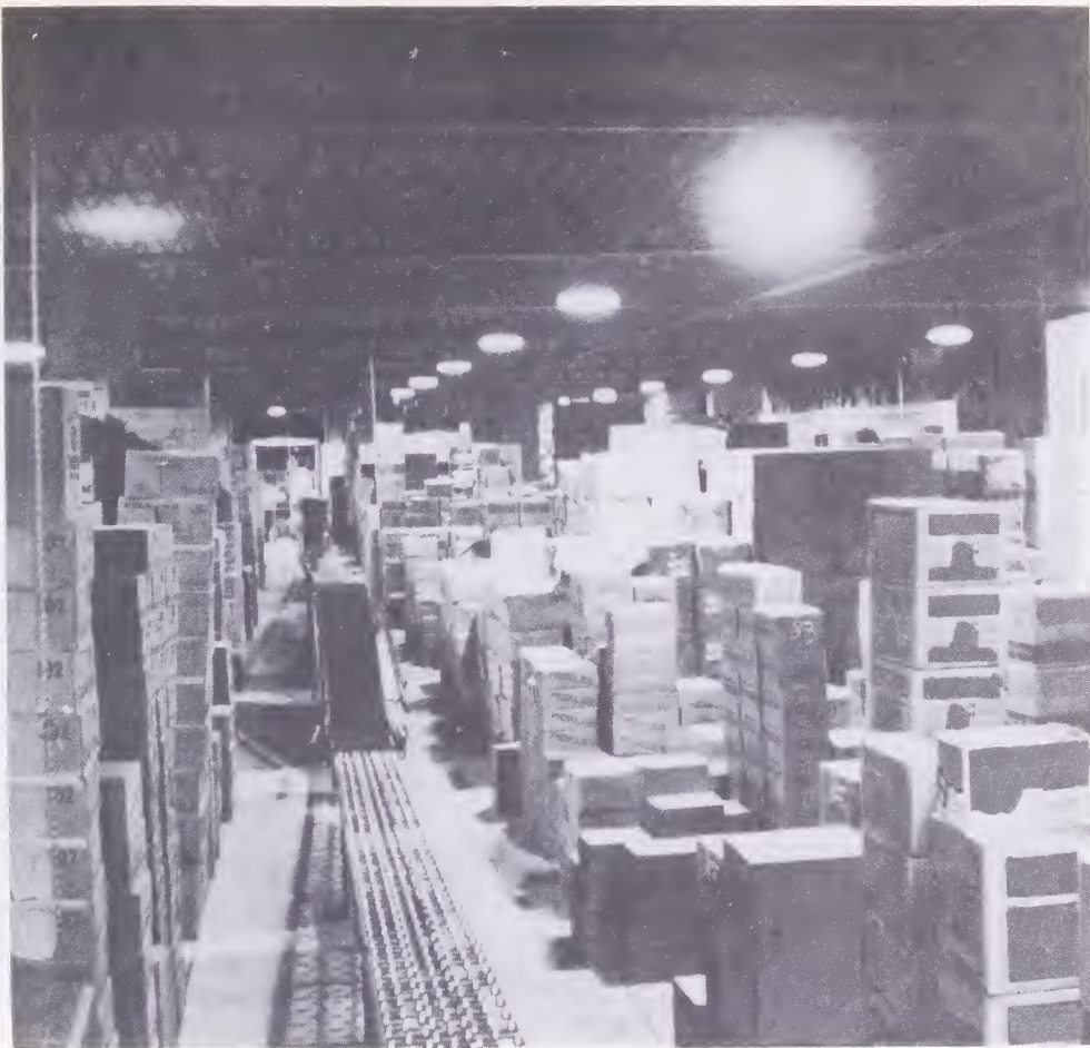
Figure 7.--A wheel type conveyor system in a 1-floor warehouse with electrically operated belt boosters to provide the necessary down-grade.
