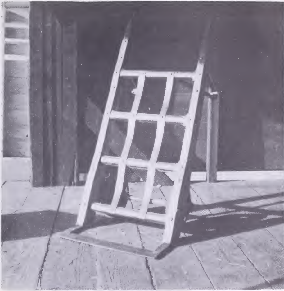
Figure 5.--A 2-wheel handtruck of the type used in some grocery warehouses for receiving and shipping merchandise.
