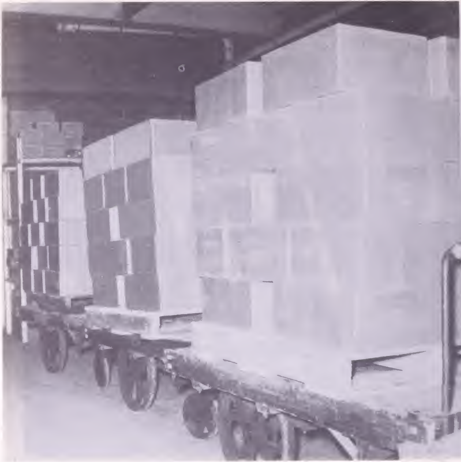
Figure 6.--A line of 4-wheel handtrucks loaded with merchandise palletized in a rail car. The palletized merchandise will be moved to storage and stacked with a forklift truck.
