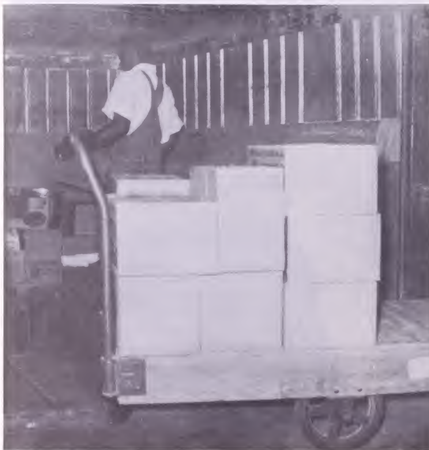
Figure 17.--A truck loader carrying cases from a handtruck into a delivery truck.
