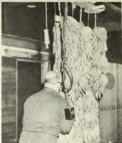
Figure 24.--A carrier of a manual monorail "ripen-on-carrier" conveyor system being moved off the lowerator and onto the fixed overhead monorail track.
