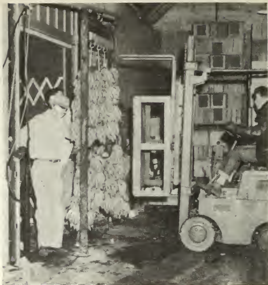
Figure 11.--Lowerator used with forklift truck system to facilitate hanging of bunches of bananas on carriers.
