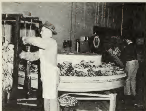
Figure 38.--Four-wheel banana truck used for positioning bunches for the cutting operation.
