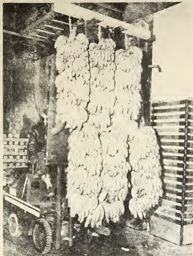
Figure 28.--Forklift truck with loaded 6-bunch carrier in position to perform the transportation operation.
