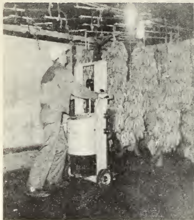
Figure 36.--Hydraulic bunch lift truck used to transfer ripe bunches of bananas from hanging position in the ripening room to the transporting equipment.
