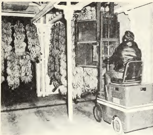
Figure 30.--Worker with forklift truck positioning a loaded 6-bunch carrier in the ripening room. Note special beams for holding the 6-bunch carrier.
