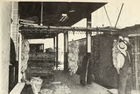
Figure 6.--Bunches of bananas being removed from refrigerator car to ripening room by use of a continuous powered mono-rail conveyor.
