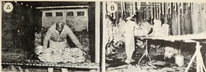
Figure 32.--Gravity-type wheel conveyor being used to move bunches of bananas from railroad car (A) to ripening room (B). (Note the plywood boards which are utilized as runners for transporting the bunches.)
