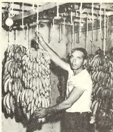
Figure 7.--Worker removing a bunch of bananas from a 1-bunch carrier on a manual monorail conveyor prior to hanging it on ceiling hook.
