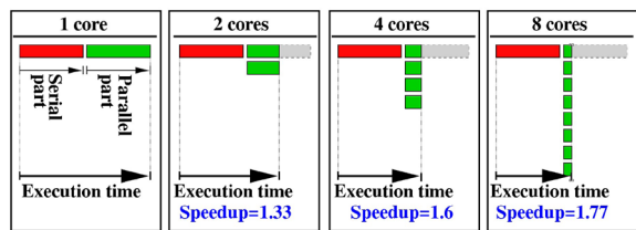
If 50% of the application is sequential, then the maximum speedup is 2 Source: own representation of the Amdahl's law (Amdahl, 1967)
