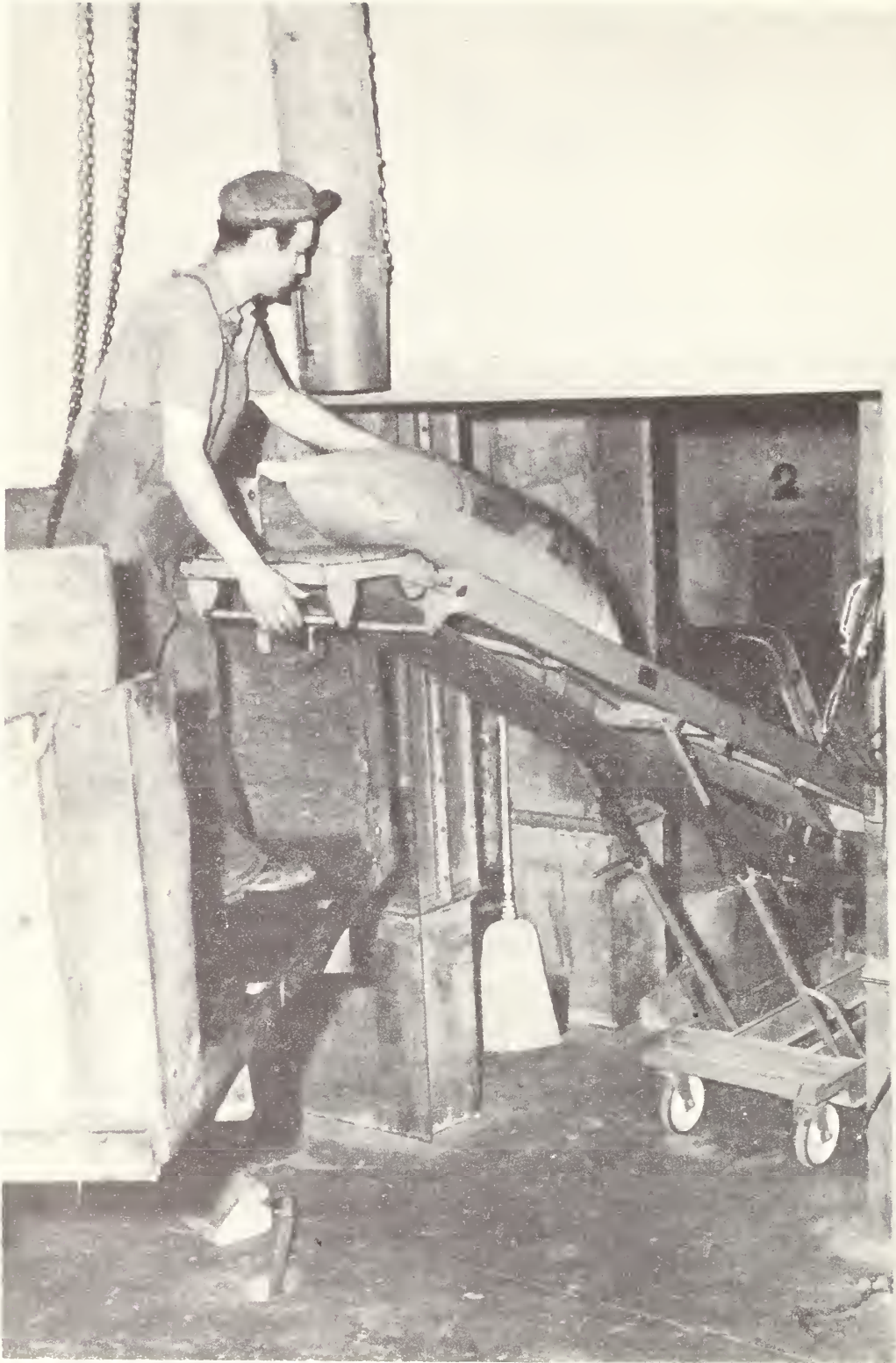
Figure 27.--Portable conveyors for bagged goods speed up handling and reduce costs of operation.
