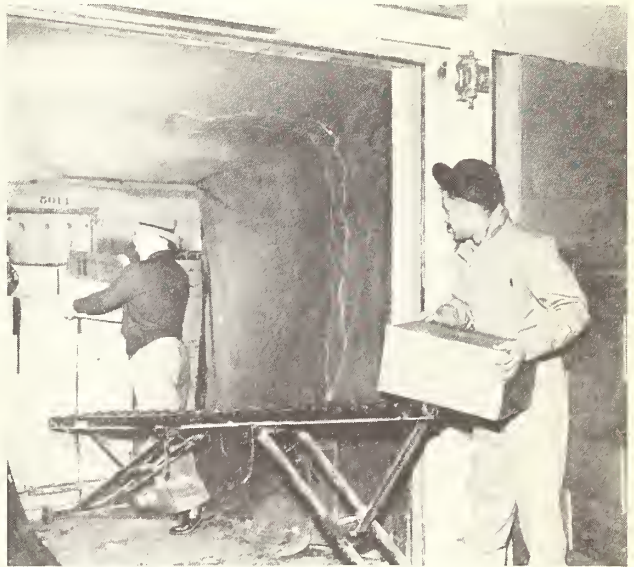
Figure 21.--Gravity conveyors can be used for performing a number of different operations at wholesale plants. However, conveyor operations are often unbalanced. The worker loading the conveyor above has to wait to send packages down the line until the worker stacking cases in the motortruck is ready to receive them.
