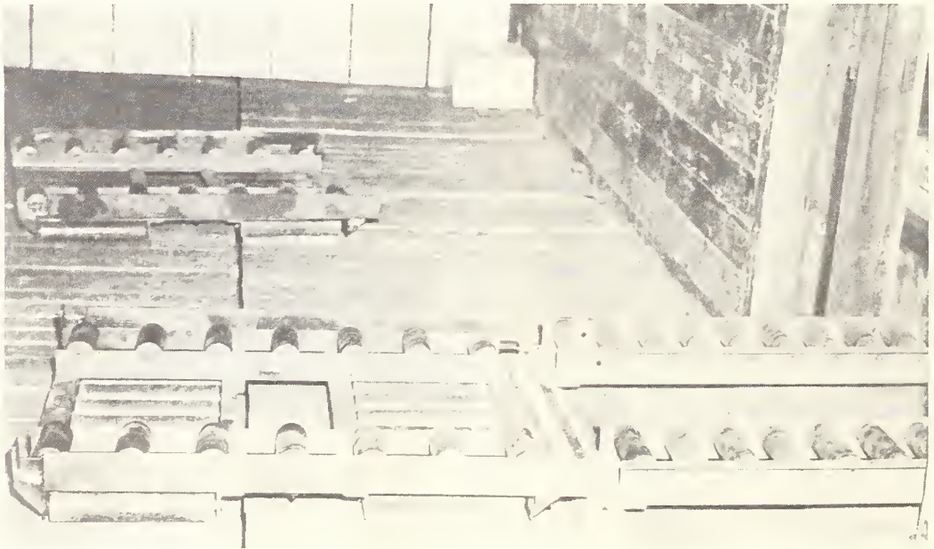
Figure 23.--Pallet dolly in position for transfer of loaded pallet to conveyor for removal from railroad car doorway by fork-lift truck.
