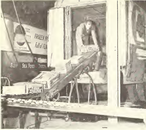
Figure 20.--Portable belt conveyors, such as the one shown, are useful for moving merchandise from a lower level to a higher one. They can be easily tied in with gravity conveyor operations.
