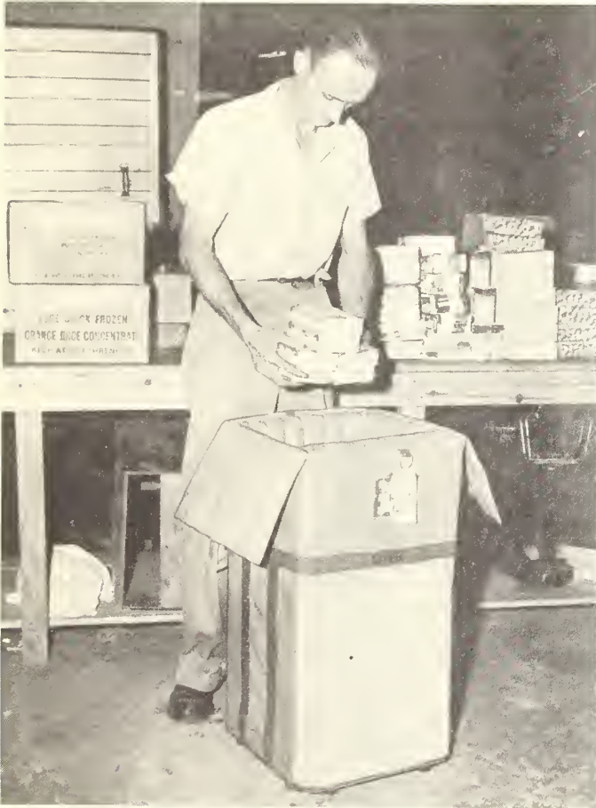
Figure 6.--Individual packages and/or full cases of frozen foods can be packed in insulated shipping containers for delivery to customers. Frozen foods in these containers can be delivered with products that do not normally require refrigeration. Dry ice is placed in the top of the container unless hauls are of very short duration. Wholesalers who make extensive use of these delivery containers should make special provisions for packing them during the order-assembly process.
