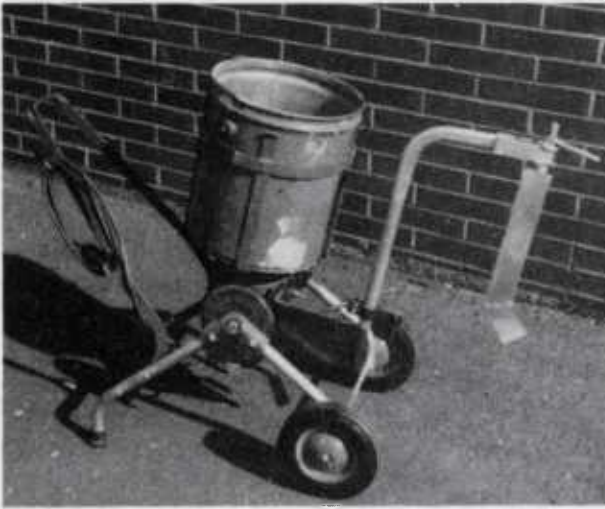
Figure 22.—Motor-driven plasterer's mixer for mixing small batches of surface bonding. The cylindrical metal container rotates against a rubber or plastic blade, creating a scraping action that does not cause the fibers to "ball up" as with other types of mixers.
