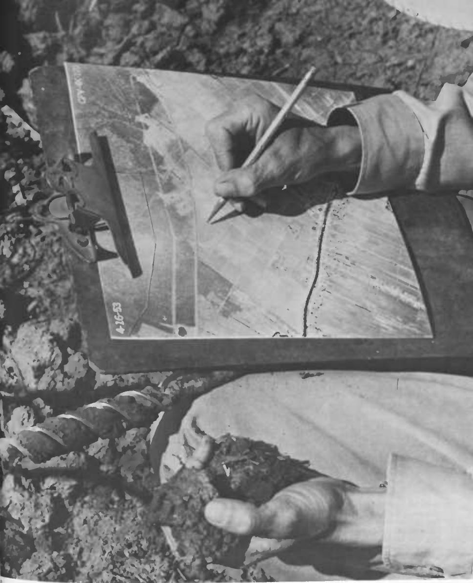
Figure 19.— A soil scientist examines the soil, identifies it, and draws its boundaries on an aerial photograph.
