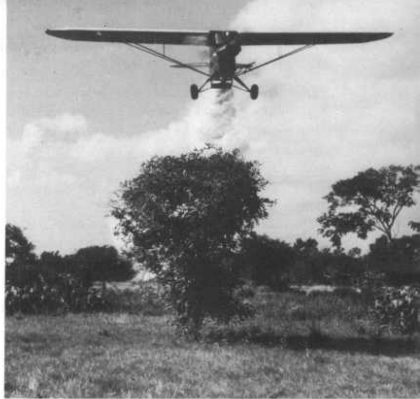
In large mosquito-infested areas, spray planes can be used for applying insecticide sprays and dusts.
