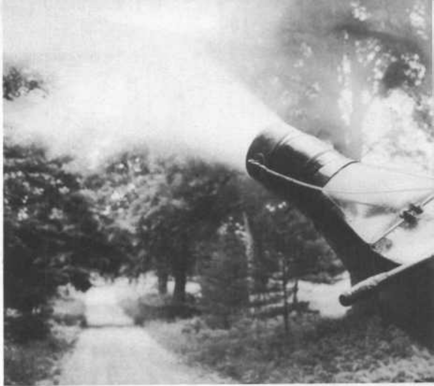
Use of a powerful mist blower mounted on a truck speeds up the task of controlling insects in trees.
