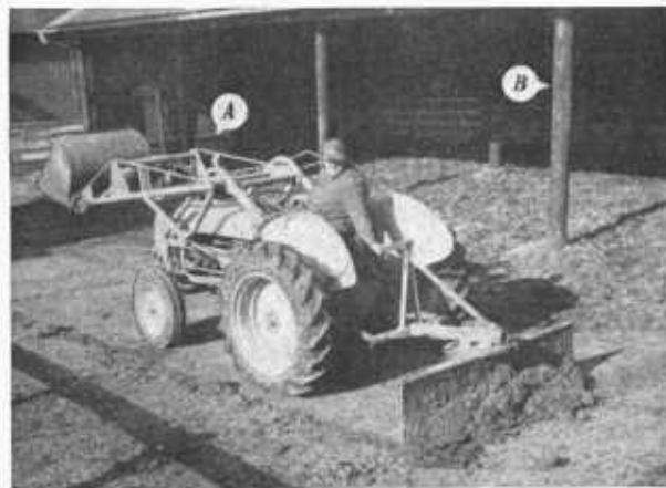
FIGURE 17.—Paved strips in front of resting areas can be easily cleaned with tractor-mounted equipment. Pole sheds should have pressure-treated retaining planks (A) and poles (B).
