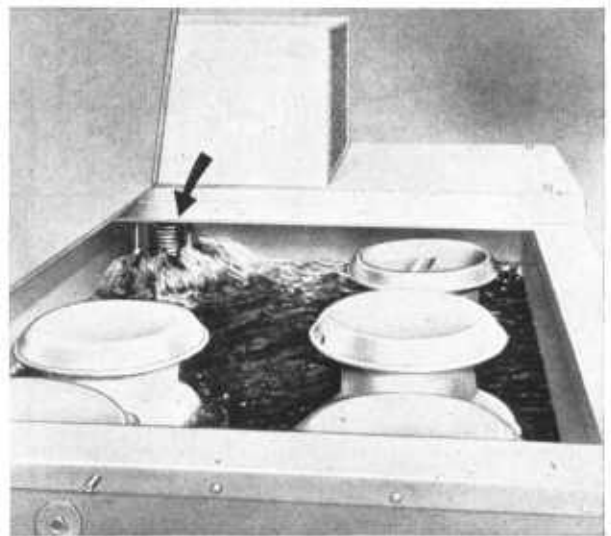
FIGURE 11.—Milk coolers of water-spray type (above) and water-immersion type (below). Immersion cooler shown has a mechanical unit (arrow) which circulates cooling water around cans.
