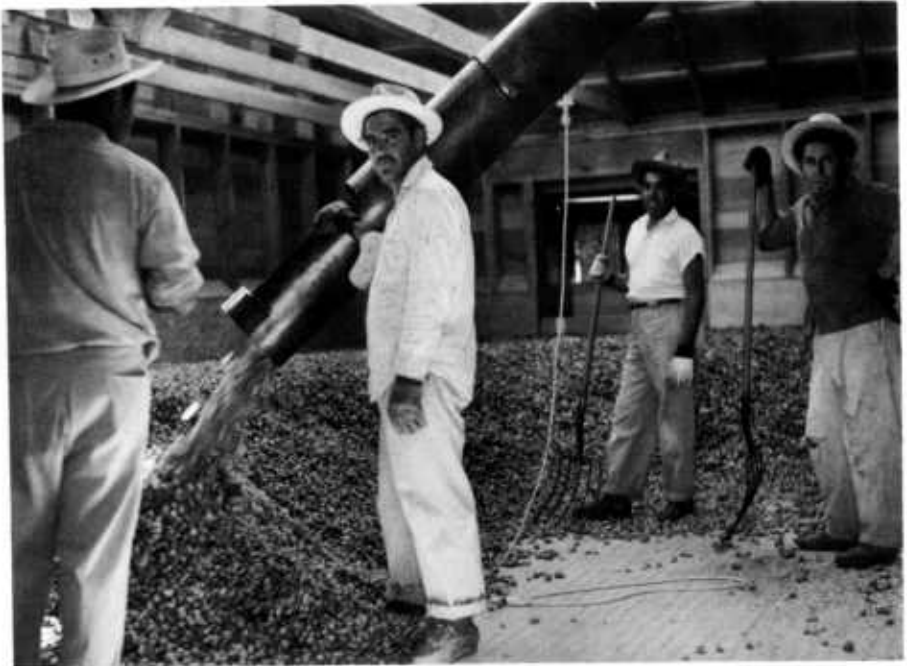
FIGURE 29.—Loading a kiln with fresh hops. Hops are carefully forked to prevent uneven packing.
