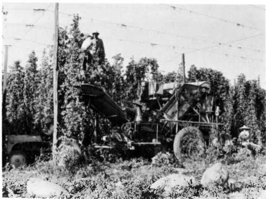
FIGURE 28.—Portable hop-picking machine.
