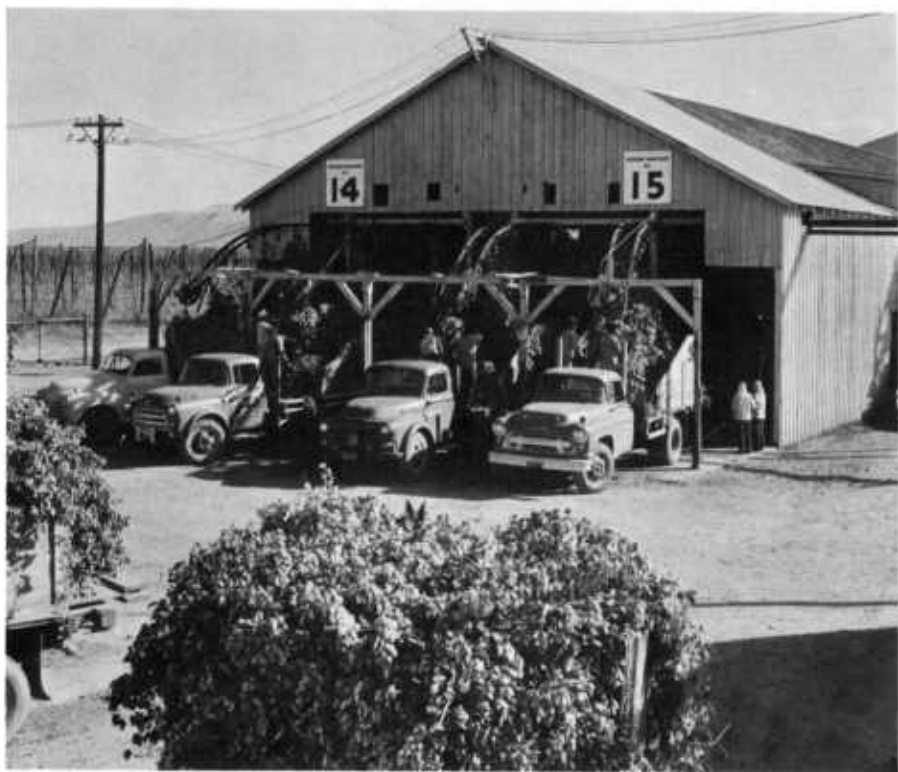
FIGURE 25.—Unloading vines from V's at picking machine and clamping them into grasper bar.
