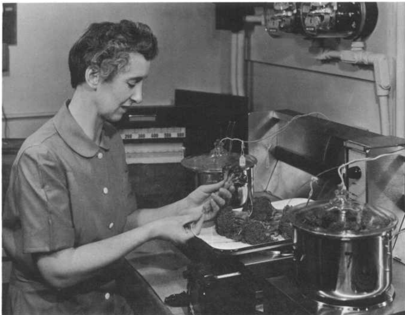
Thermocouples measure heat penetration in broccoli in studies to determine the best methods of cooking to maintain or enhance eating and nutritive quality.
