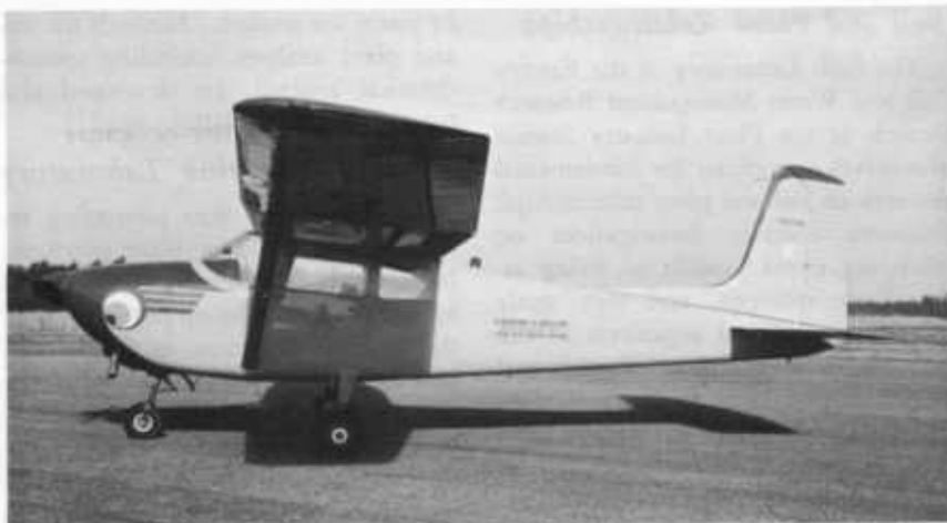
An airplane used in plant pest-control research. Equipment on plane can be adapted to solve changing problems in dispersal of agricultural chemicals.
