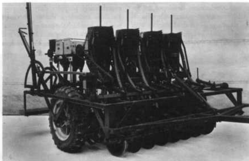
Drill designed for grassland-establishment experiments on prepared seedbeds or for plot work with grains. Fertilizer and seed may be broadcast and drilled or planted at different depths and spacings.
