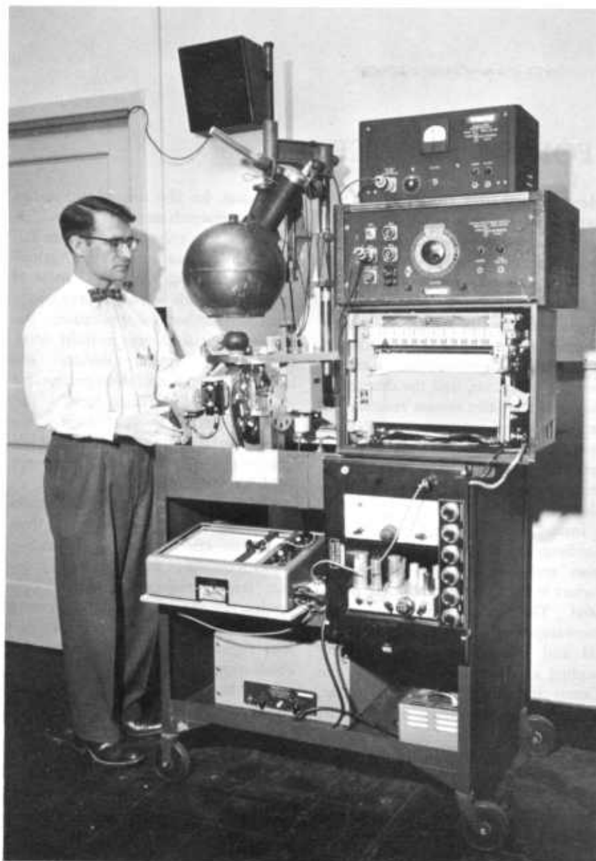
An engineer measures the interior color of a tomato with a special instrument developed by Department research workers. This instrument records the light-transmittance properties of intact fruits and vegetables.
