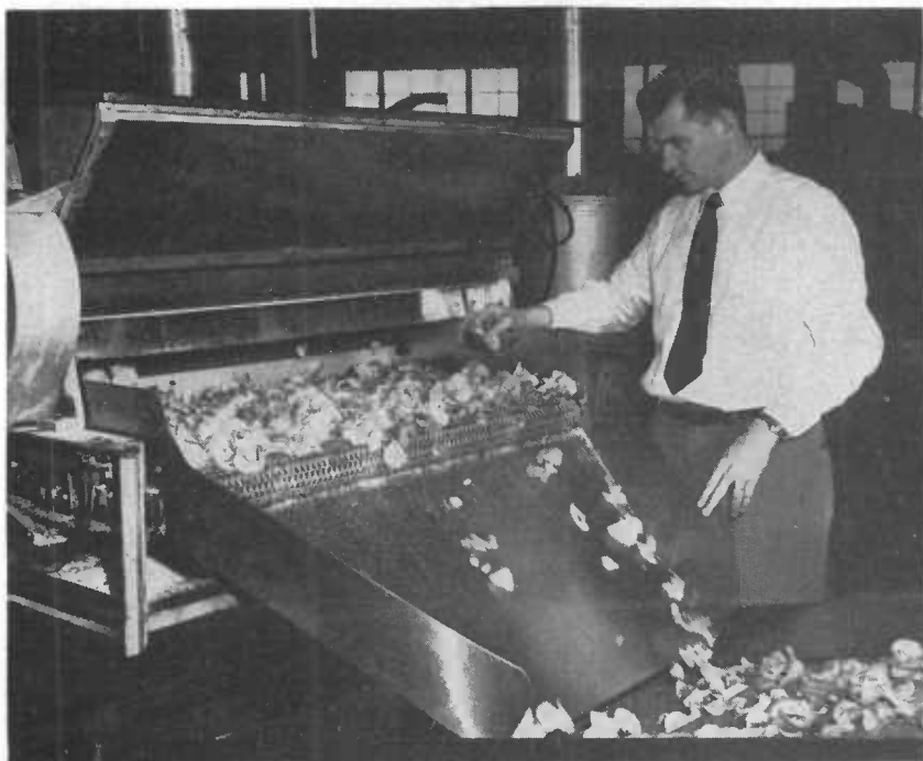
FIGURE 1.—Potato chips as they leave the fryer. An automatic conveyor carries the potatoes to the peeler, to the slicer, and then through the fryer.
