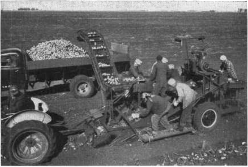
FIGURE 7.—A mechanical harvester in operation in the Red River Valley. The workers riding on the harvester are removing vines and trash as the potatoes are elevated into the truck.
