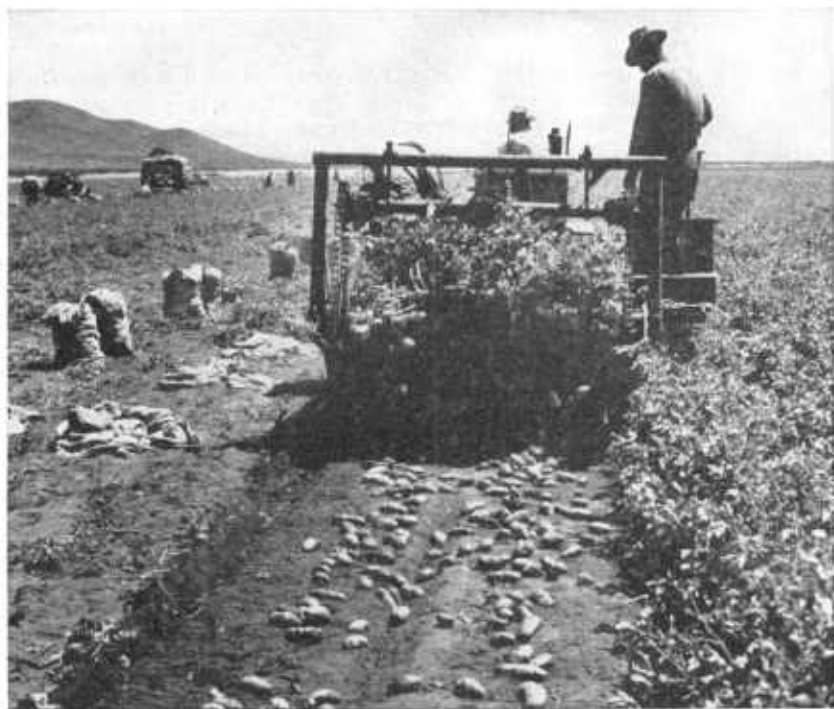
FIGURE 5.—A two-row, level-bed digger in Kern County, Calif. The man on the digger adjusts the depth of the digger blade and removes vines that clog the digger chain. In this area field sacks are used in hauling the potatoes to the packing shed.
