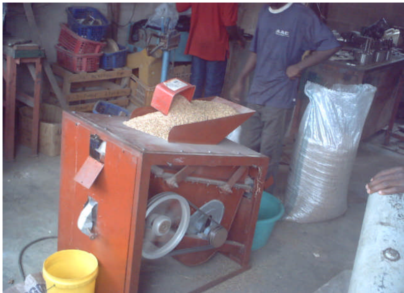
Hanigha de-stoning machine in operation (the green & yellow buckets collect de-stoned paddy & stones,
