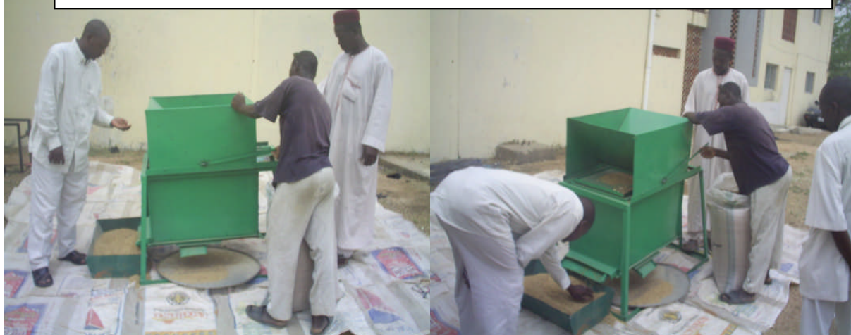
Locally fabricated manual de-stoner being operated at Dandago Agro-machinery
