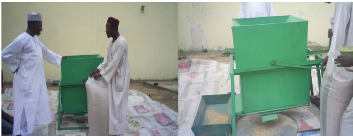
Locally fabricated manual de-stoner being operated at Dandago Agro-machinery
