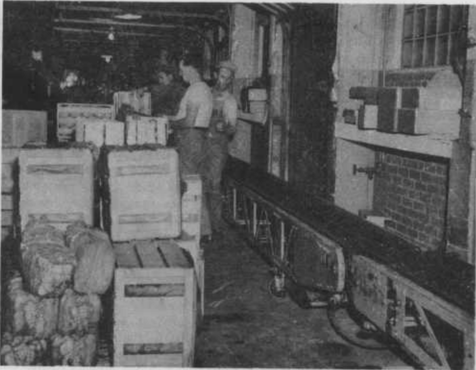
Figure 7.--Checker calling items. Note laborer working with him and lateral belt conveyor on the right. Man in background is assembling the next load and is not a member of truck loading crew.
