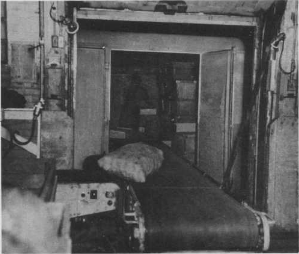
Figure 6.--Cantilever belt conveyor, extended into the body of the motortruck, being fed from one of the reversible lateral belt conveyors. Note 100-pound bag of potatoes being automatically transferred from lateral conveyor to cantilever conveyor.
