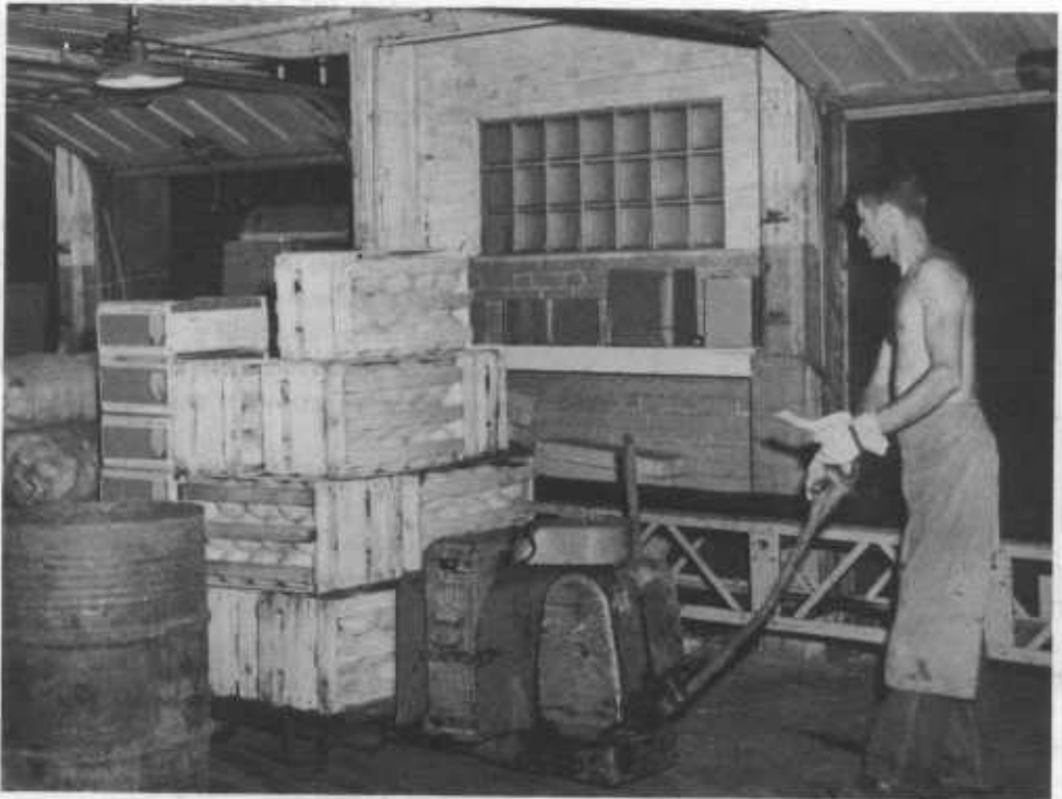
Figure 4.--Assemblyman depositing a skid load of items which have been picked from stock in conformity with the recap at the assembly point alongside the belt conveyor.
