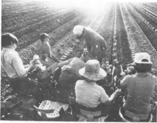
Transplanting flue-cured tobacco in ridged rows. This two-row transplanter requires four people on the machine.
