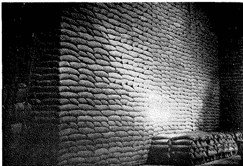
FIG. 30.—Storage of sugar in sacks. In some factories, part of the sugar is stored in bulk and later placed in sacks.
