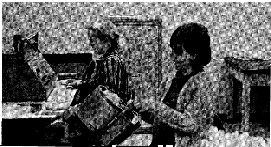
Fig. 15. Modern laboratory equipment, such as this digital fibrograph, has improved the accuracy and speed in evaluating cotton strains.
