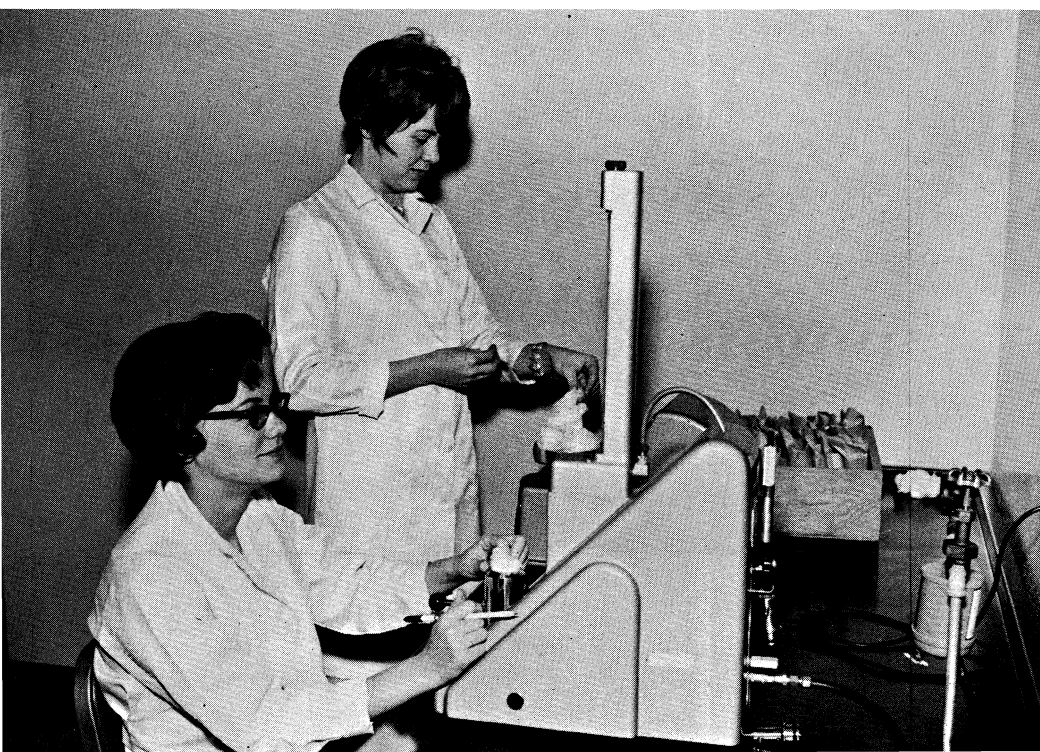
Fig. 17. The micronaire, which measures fiber maturity and fiber fineness, has become an important tool for selecting desirable cottons for the irrigated Southwest.
