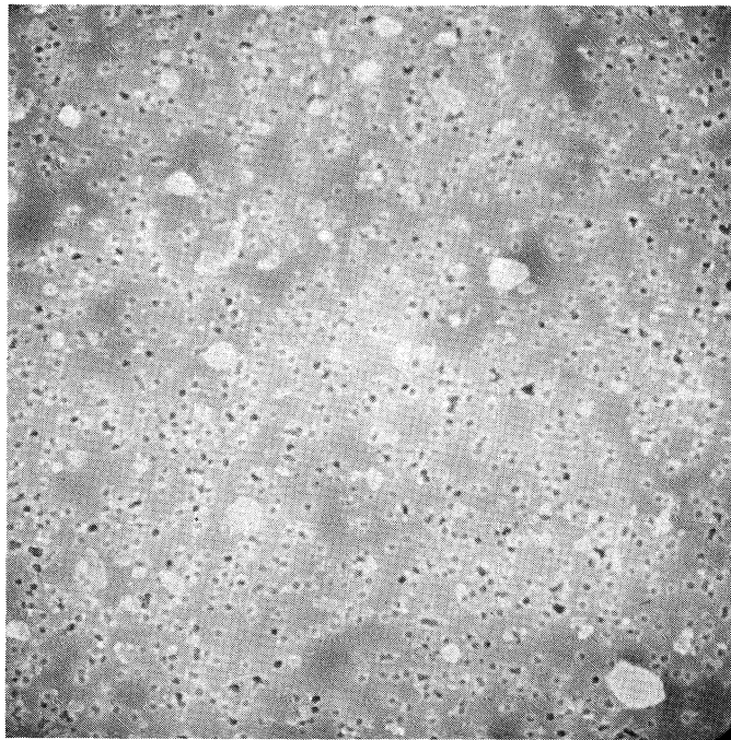
Figure 16. Filter Surface after Long Extraction Interval
