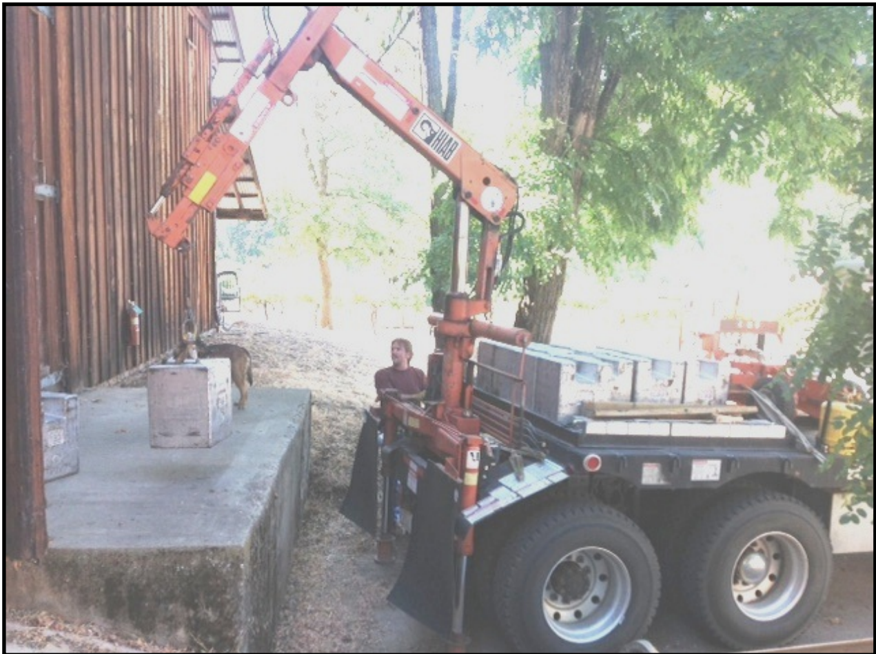
Steve Farris, Calaveras County Agricultural Technician, uses the weight truck crane to unload 1,000 pound standards at Rorick Vineyard for testing of their bulk grape platform scale.
