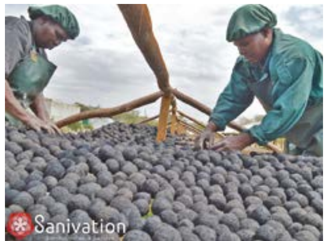
FIGURE 2.3. (A) PROCESSING BRIQUETTES IN KAKUMA USING AN AGROMERATOR, (B) BRIQUETTES BEING DRIED IN KAKUMA, (C) PACKAGED AND BRANDED BRIQUETTES, (D) BRIQUETTE BURNING.
