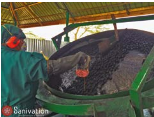
FIGURE 2.3. (A) PROCESSING BRIQUETTES IN KAKUMA USING AN AGROMERATOR, (B) BRIQUETTES BEING DRIED IN KAKUMA, (C) PACKAGED AND BRANDED BRIQUETTES, (D) BRIQUETTE BURNING.
