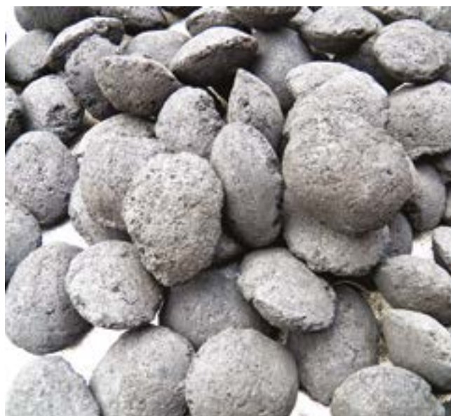
FIGURE 3.1. PILLOW-SHAPED FUEL BRIQUETTES.
