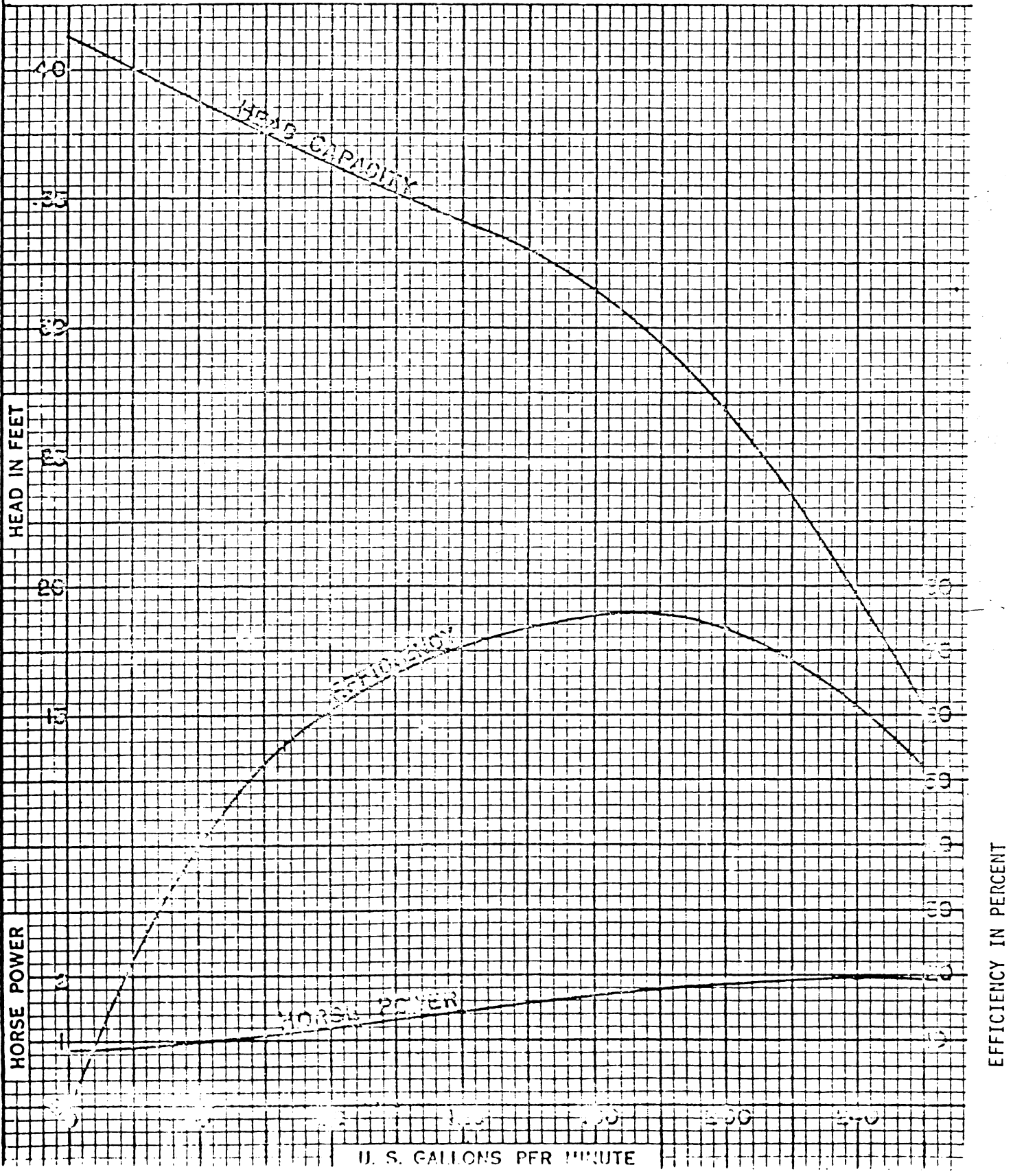
Figure 3-2: Official Efficiency Curve for Representative Pump Operating With One Stage.
