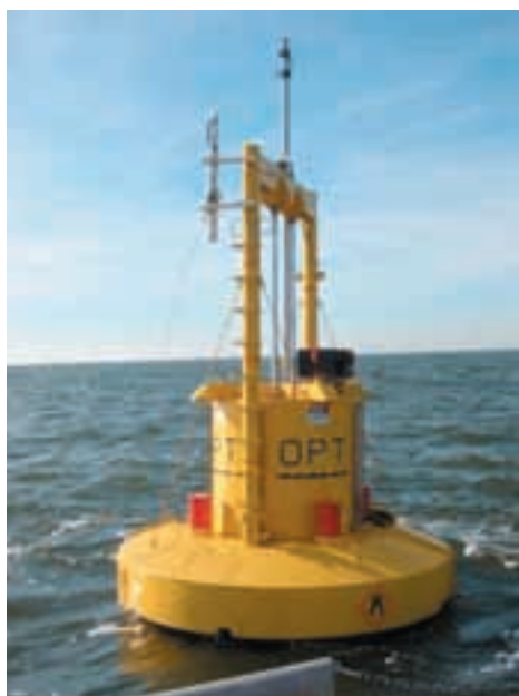
PNGC will be using huge buoys such as this to harness the power of ocean waves off the coast of Oregon. Photo courtesy PNGC
