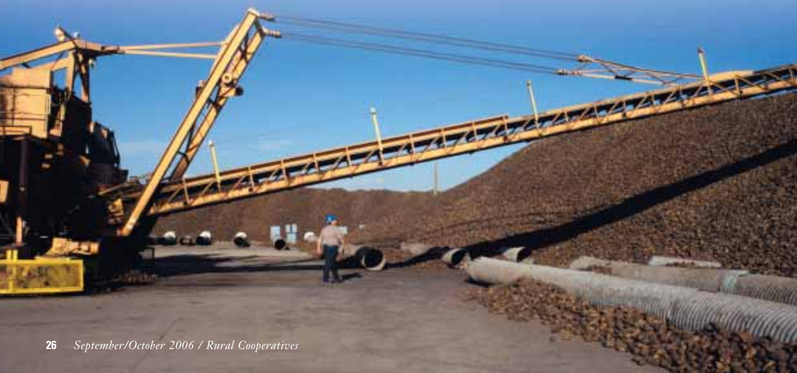
Sugarbeets thrive in the rich soil of the Red River Valley of Minnesota and North Dakota. Photo courtesy American Crystal Sugar (ACS); A conveyor transports sugar beets from stockpiles into the ACS processing plant in Moorhead, Minn. USDA photo by Dan Campbell
