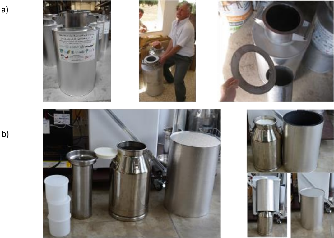
Figure 9: Insulated milk can concept a) initial design and b) improved design
