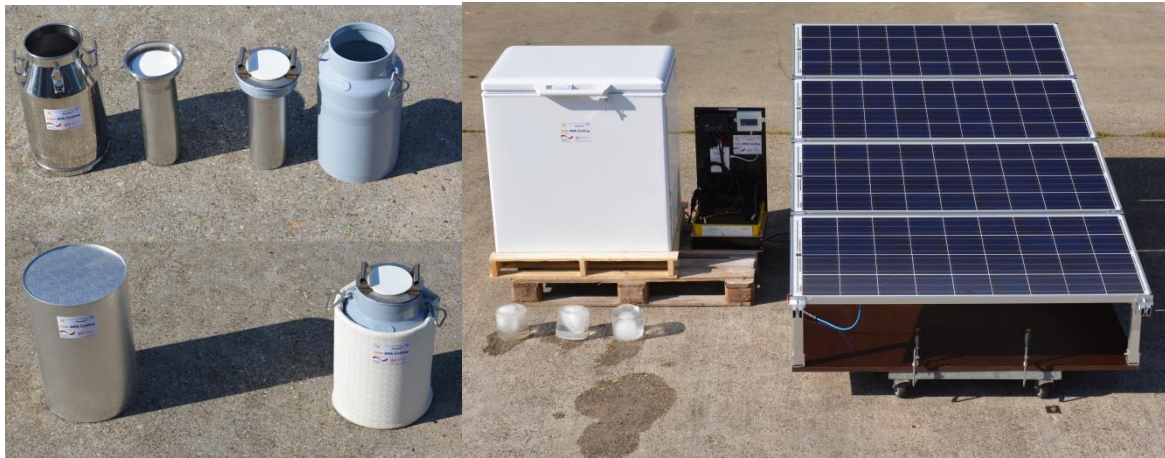
Figure 1: Solar milk cooling components a) insulated milk cans and b) PV modules control panel and DC freezer
