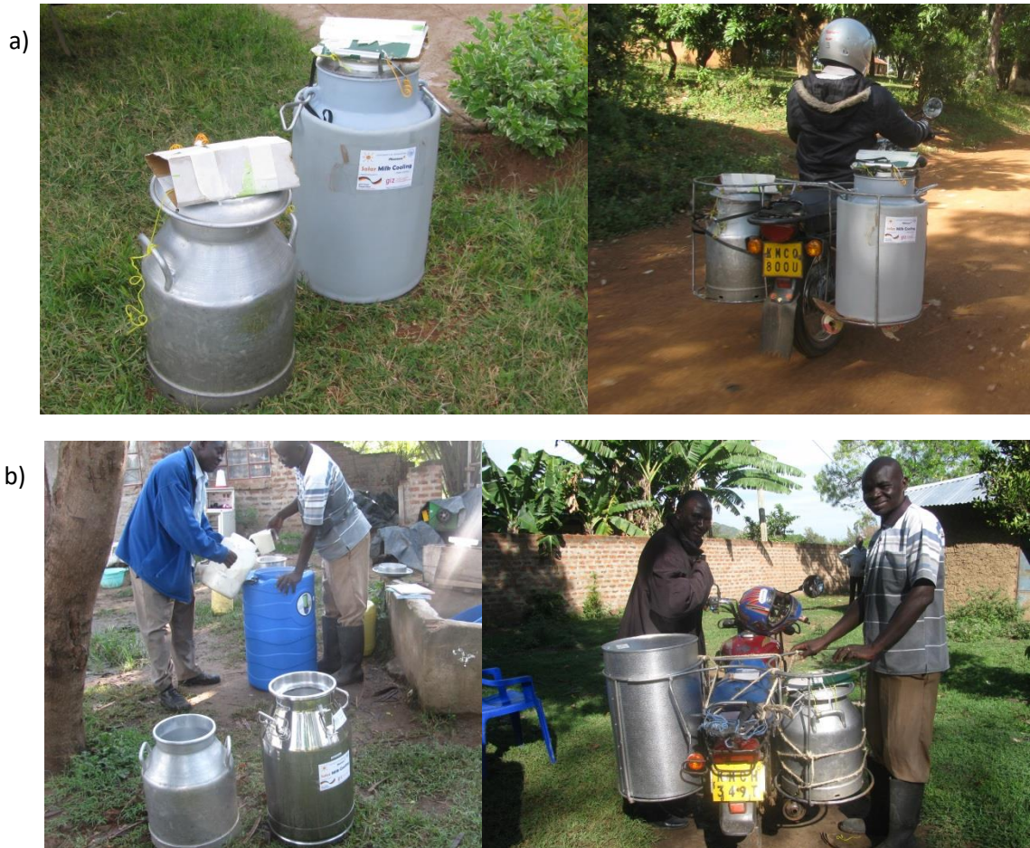
Figure 15: Transport of the modified milk cans a) Plastic-prototype and aluminium milk can (control condition) and b) Stainless steel-prototype and aluminium milk can (control condition)
