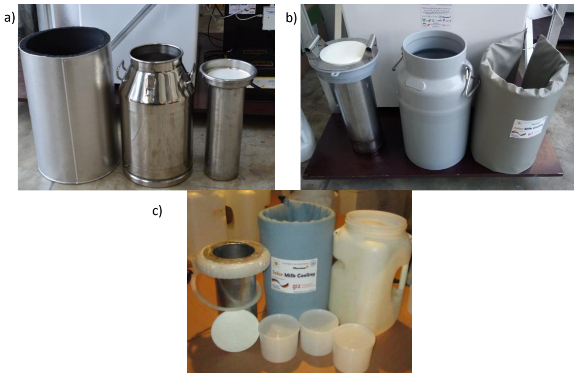
Figure 5: Modified milk cans a) 40l stainless steel milk can, b) 40l plastic milk can and c) 10l plastic milk can (Mazzi can)
