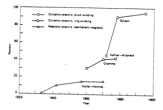
Efficiency of electric generators: electric power output per unit of mechanical power input.
