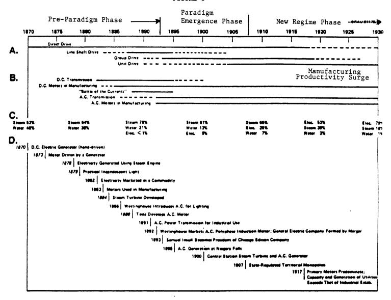
Chronology of electrification of industry: (A) Methods of driving machinery; (B) Rise of alternating current; (C) Share of power for mechanical drive provided by steam, water, electricity; (D) Key technical and entrepreneurial developments.
