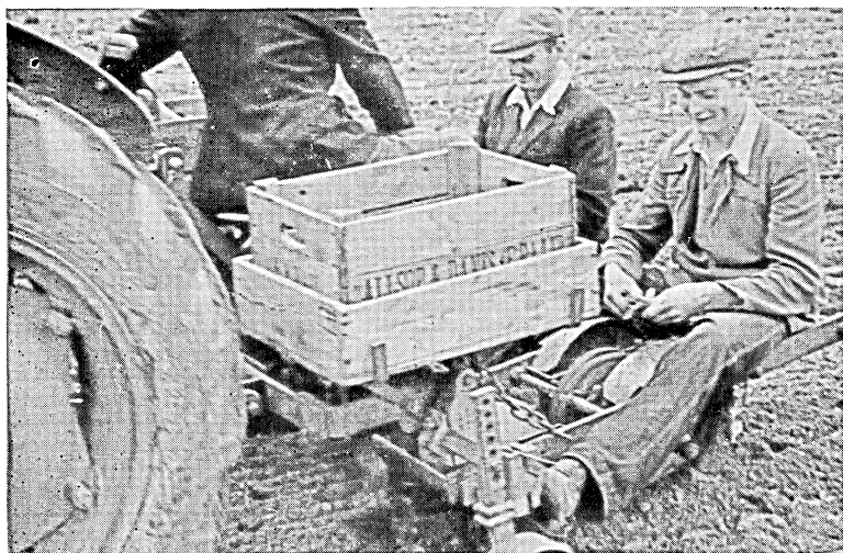
PLATE XVI. The use of the 'easy-feed attachment' provides greater comfort for the planters.
