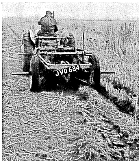
PLATE XIX. A semi-mechanical method ; the carrots are picked up by hand behind the lifter.
