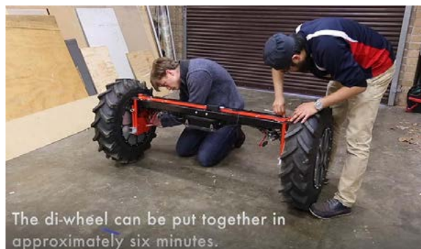
Figure 6. Two people can quickly attach the expandable central shaft with its sensors.
