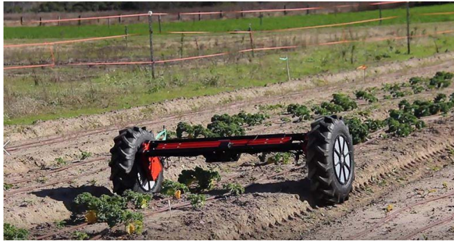
Figure 7. Trial of the di-wheel adjusted to width to scan a row of vegetable crop.
